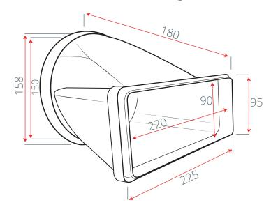
Ducting – Our slimline motor is designed with a rectangular ducting system. Please note as this ducting is rectangular and not round, it will have different dimensions.
